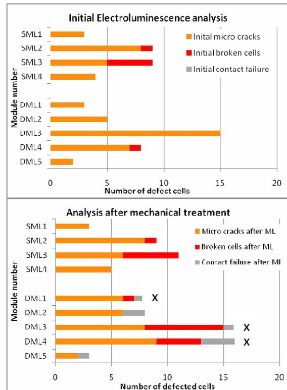
**Figure 2:** Micro cracks, broken cells and contact problems before and after mechanical load tests, detected via electroluminescence. X indicates those modules that showed a total power loss after mechanical load.
