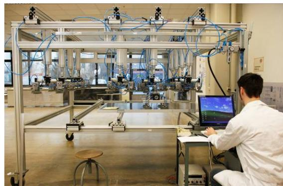
**Figure 1:** Mechanical load set-up at PI Berlin.
