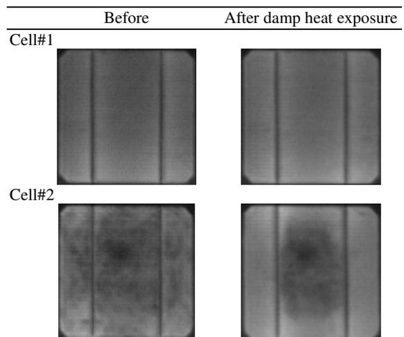
Moreover, Table IV is demonstrating as well that the passivation effect deriving from the damp heat treatment is not affecting all cells at the same level. The electrical mismatch between the cells in the same module will increase from this cell dependent passivation effect. This results in a fill factor increase as known for non-uniform
