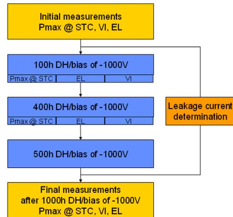
**Figure 1:** Testing scheme for our TCO corrosion test incl. leakage current determination. After 100, 400, and 500 hours (total: 1,000 hours) visual, electroluminescent and electrical results are determined
