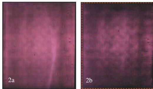
**Figure 2:** EL pictures of module Type A (a-Si, framed). 2a: initial EL-picture, 2b: EL-picture after 1,000 hours of BDH, which shows reduction of active area.
