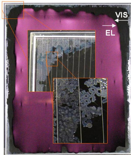
**Figure 4:** Electroluminescence picture as an overlay of the visual picture of module Type B. “EL” is marking the boundary of the active electroluminescent area to the deactivated area (22%). The “VIS” picture is showing the corroded area at the edges of the module (6.5%) with more details in the in-set images outlined in red.
