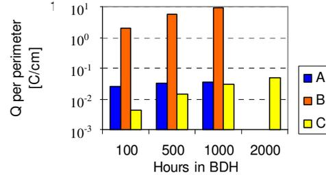
**Figure 7:** Charge  $Q$  per perimeter for biased damp heat for the silicon thin film modules.
