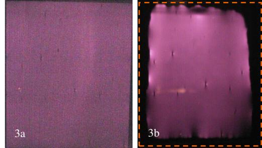
**Figure 3:** EL pictures of module Type B ( $\mu$ -Si, laminate, fixed with clamps):
