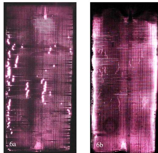
**Figure 6:** EL pictures of module Type D (CdTe laminate, fixed with clamps). 6a: initial EL-picture, 6b: EL-picture after experiment showing new shunts developed at the module edges on the left and right side.
