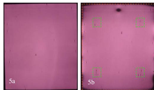
**Figure 5:** EL pictures of module Type C ( $\mu$ -Si, laminate, fixed with special mounting fixtures at the backside). 5a: initial EL-picture, 5b: EL-picture after biased damp heat shows reduction of active area and new shunts, marked with green rectangles, developed in the area of the mounting fixtures.
