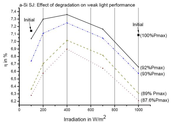
**Figure 9:** Weak light performance (100 to 1000 W/m<sup>2</sup>) at different degradation levels for a single junction a-Si module (a totally degraded module of this type would show 75% of the initial power  $P_{max}$ ).
