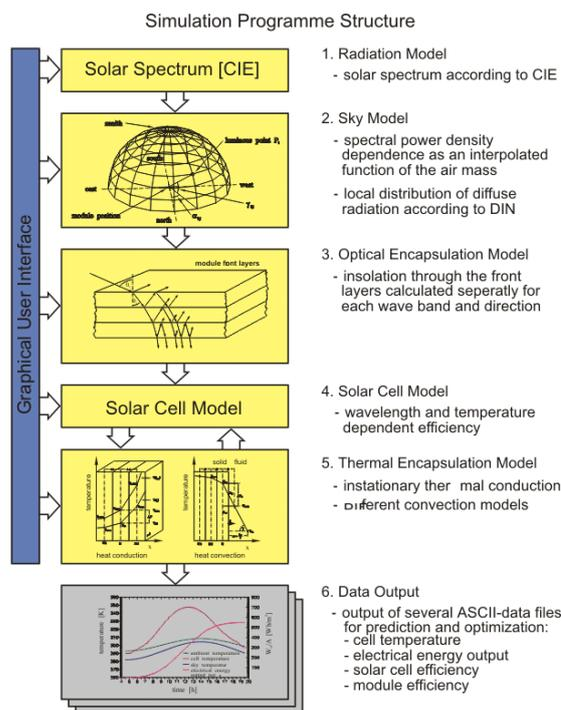
**Figure 1:** Structure of the PV yield prediction software.
