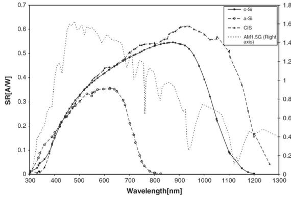
**Figure 2:** Comparison of absolute spectral responses for different solar cell materials, together with an AM 1.5<sub>G</sub> spectrum (according to [9]).
