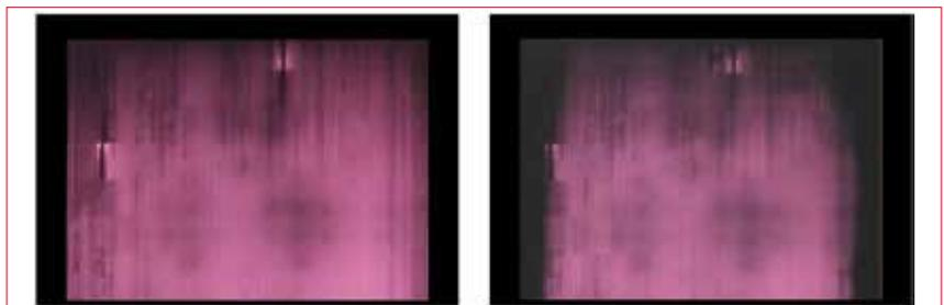
Figure 4. EL photography applied to a-Si modules, showing initial state (left) and after 1000h of damp-heat treatment (right – considerable reduction of photovoltaic active areas due to TCO corrosion (see TCO corrosion section overleaf).
