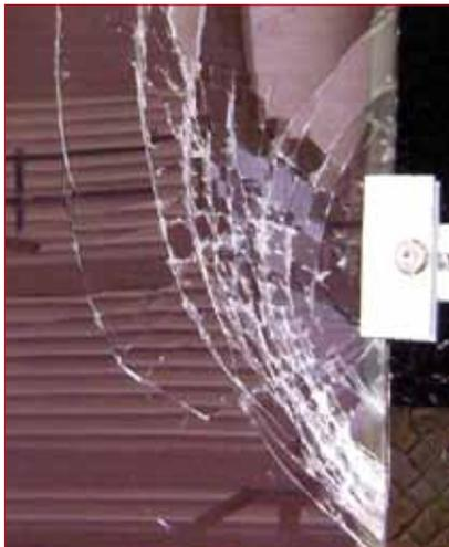
Figure 1. Breakage at 2,400 Pa: a-Si 1.4m<sup>2</sup> module with 2mm x 3mm glass.
